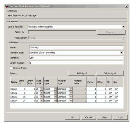
• CANdb specified signals: Allows you to specify a CAN database file that contains message and signal definitions. If you select this option, select a CANdb file. The number of input ports on your block depends on the number of signals specified in the CANdb file for the selected message.
