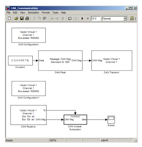
The CAN Configuration block does not connect to any other block. This block configures the CAN channel used by the CAN Receive block to receive the CAN message.
