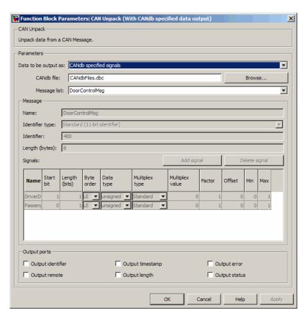
The number of output ports on your block depends on the number of signals specified in the CANdb file. For example, if the selected message in the CANdb file has four signals, your block has four output ports.
