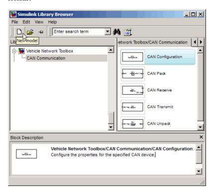
You can also select **File > New > Model** from the Simulink Library Browser. Simulink opens an empty model window on the display. To name the new model, use the **Save** option.
