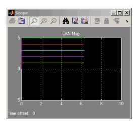
If you cannot see all the data on the graph, click the Autoscale toolbar button, which automatically scales both axes to display all stored simulation data.
