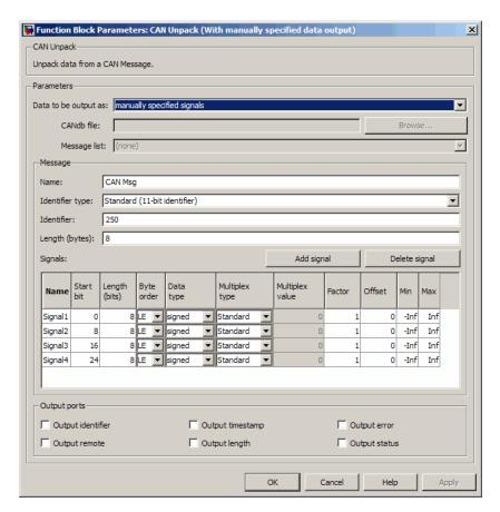
The number of output ports on your block depends on the number of signals you specify. For example, if you specify four signals, your block has four output ports.
